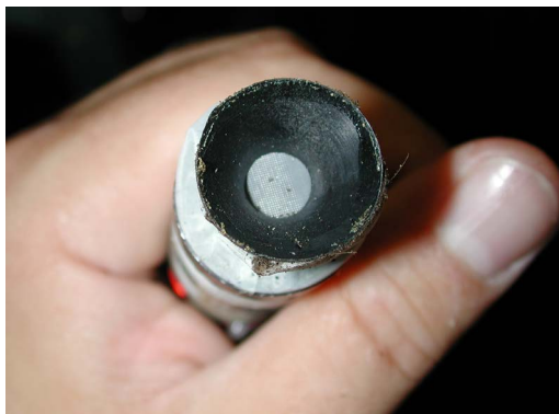
Figure 37: cone with foam remains on the edge
