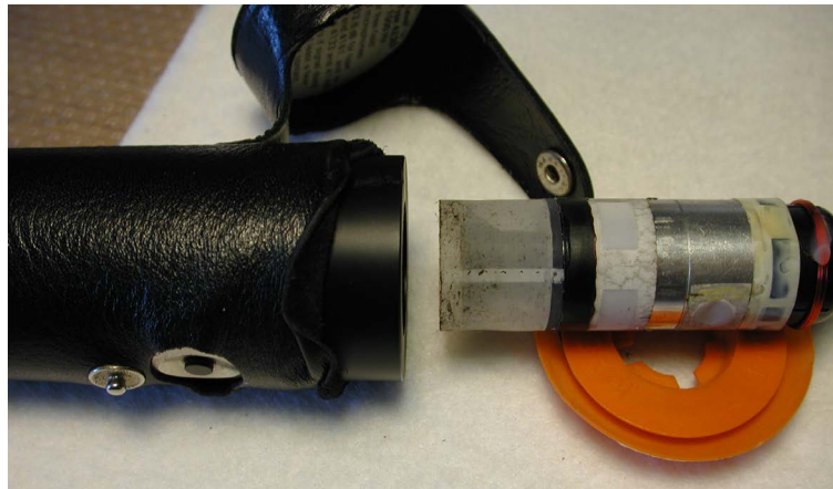
Figure 29: Sound calibrator with 94dB(A) on the microphone capsule
