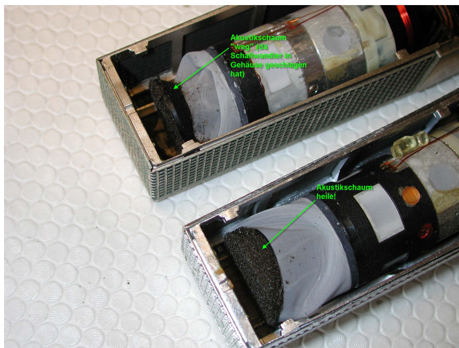
Figure 5: top: compressed acoustic foam. bottom: fixed
