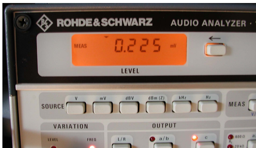
Figure 30: output voltage of the electroacoustic transducer with 94dB(A) into the speech input basket
