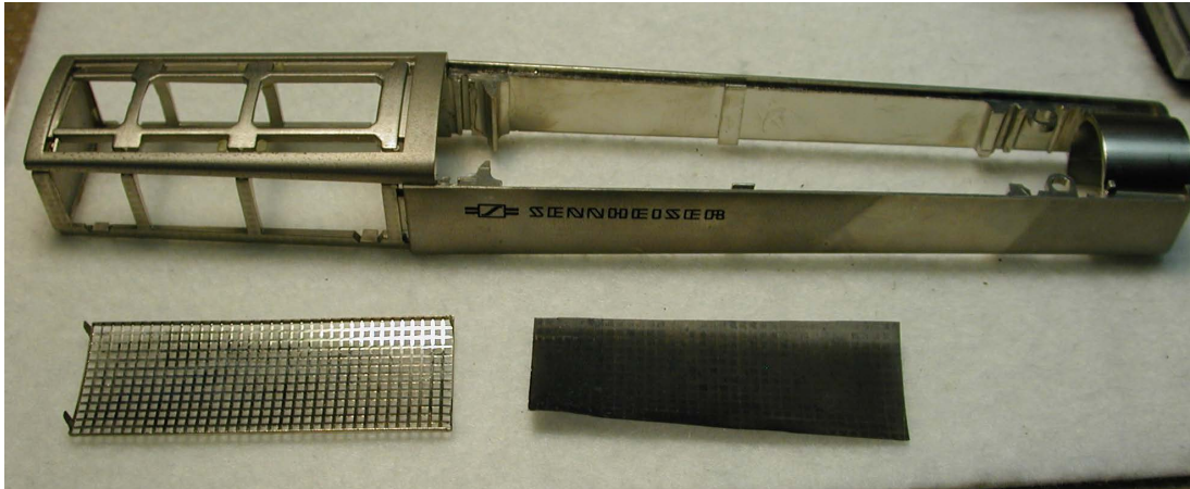
Figure 19: MD-441 frame and speech input basket with metal gauze
