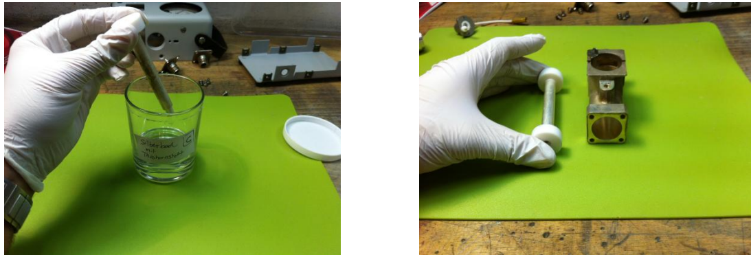
figure 21: using chemical silver cleaner for the RF path
