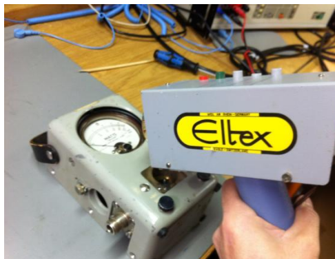
figure 7: using an ESD gun for electrostatic measurement
