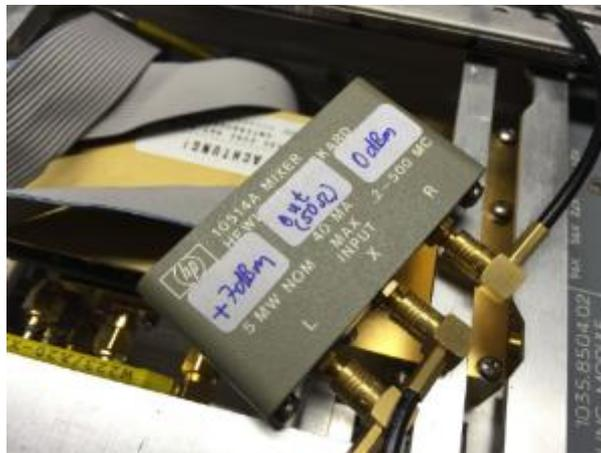
**Abbildung 3: Double Balanced Mixer HP10514**
